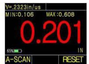
Min./Max.modes, reading in red means alarm
